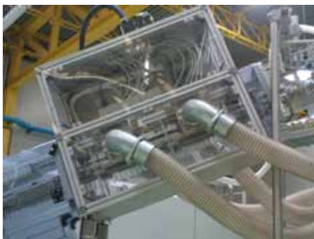
Filtered air flow to clean preforms before blowing
