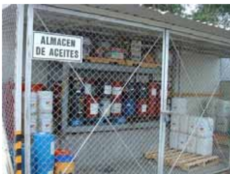
Separate and ventilated storage area for chemicals
